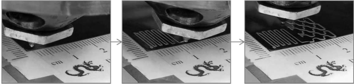
Figure 2-3: Macro-scale patterning of printed PCL square wave and sinusoid patterns by precision extrusion deposition.
